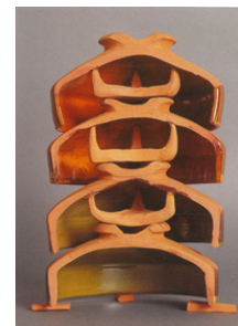
Fig 1. Cross-section of bowls in the kiln showing tripod stilts (image from The Fitzwilliam Museum)
